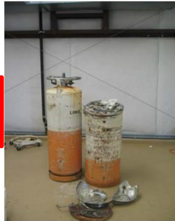
Figure 1 -Effect of Explosion on Dewar Cylinder Compared to unaffected cylinder
