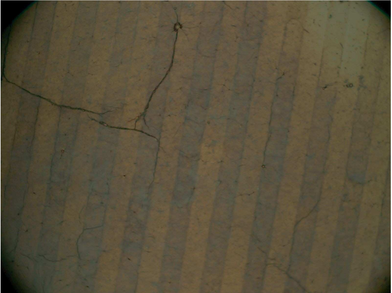
Figure 1: Mimic-based patterning on GO film with Ascorbic Acid treatment using a 20 micron channel size stamp.
