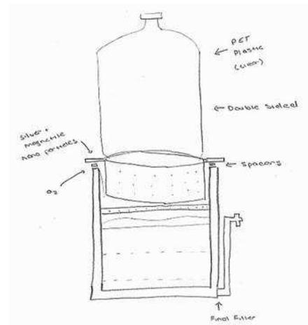
Figure 4: Household Biosand Filtration System
