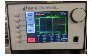
When using the Inficon controller during remote mode you need to select a process that uses the Organic source. For this example the organic source is source #3 as shown in the first picture.
