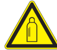
Pressurised gas hazard
